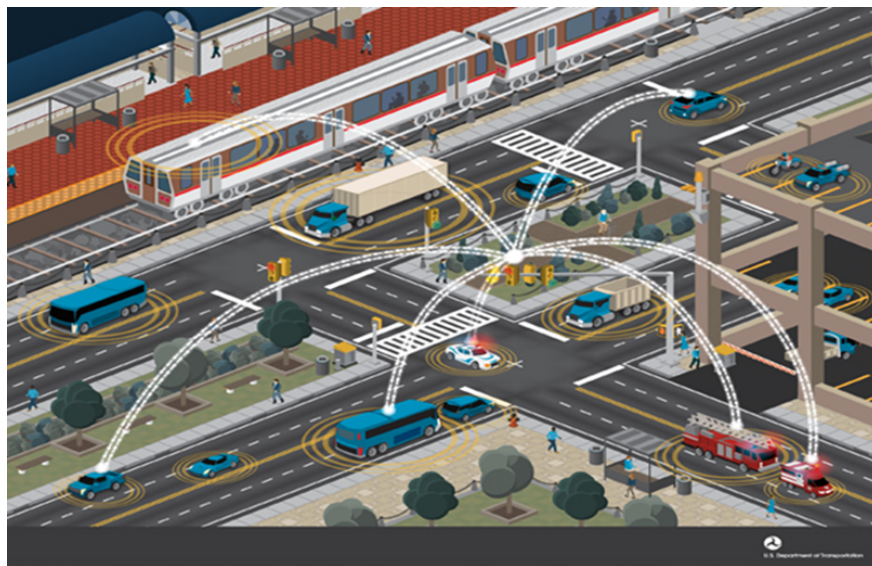
Figure 14. Structure of V2X communication
