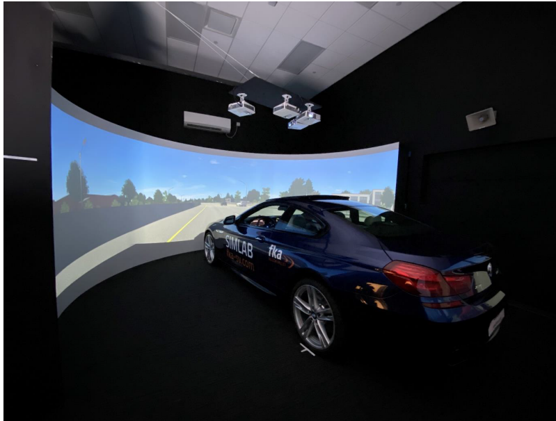
Figure 31. Hardware-in-the-loop simulator setup.
